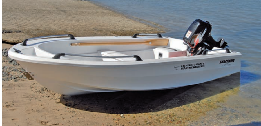
Only roto-moulding can produce a sleek design such as this in such a small craft.
